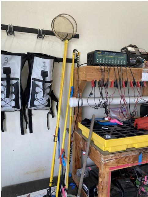
**Electrofishing Equipment: Rod ~5 lbs.; between 100 & 500 volts, Electrofishing Backpacks (not pictured): Light Backpack ~ 20 – 25lbs; Heavy Backpack ~ 25 – 30lbs Backpacks worn up to 3 hours during 8-hour shift**
