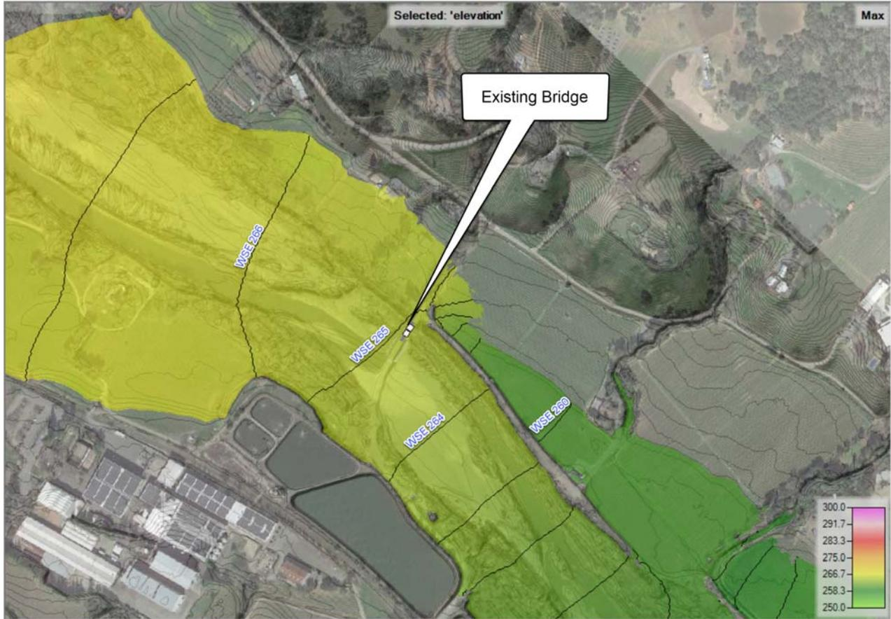
**Figure 13. Water surface elevation results for existing conditions**
